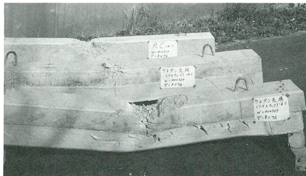
写真-2 Comparison of failure mode from upper side to lower side Type-A, C, B (W=3920N, V=8m/sec)
